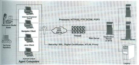
Fig. 1 A typical Performance Test Environment setup for Web Applications
