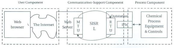
Fig. 1: Secure Internet-Based SCADA Architectural Components
